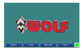
As long as no measurement data is available, the logo is displayed in the background. If measurement data is available, the last measurement value and the statistical values of the last measurement series are displayed. Operation display (bottom-right) shows the current status of the measuring device. (Green -> ready for a measuring task / Red -> measuring device is in an active measurement)
