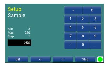
The numeric input consists of the buttons Set/</>/Exit, a numeric keypad and the parameter display. The meaning of the buttons:
