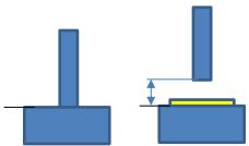
**Dwell time** = how long the measuring sensor should dwell on the object to be measured until the measured value is recorded. (the correct values are stored in the corresponding standards).
