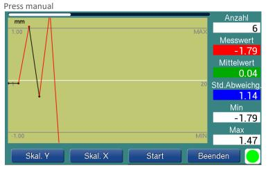
This is the access point for manual measurement. The individual measurement is triggered with Start (or by pressing the foot-operated switch). The display is graphical and numerical. The scaling works as described for the automatic measurement. To return to the main menu, press "Exit". SWITCH
