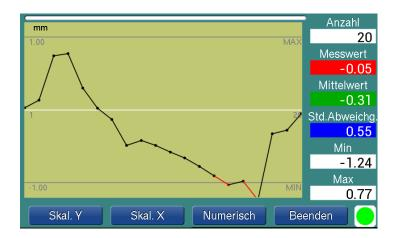
The automatic measurement is started immediately. A submenu with *Scal. Y / Scal. X / Numeric / Exit* controls the graphical display or is used to stop the measurement.
